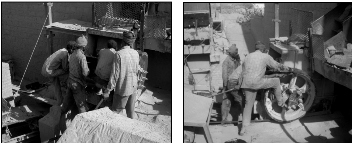
Picture 17; maintenance and cleaning of crusher
