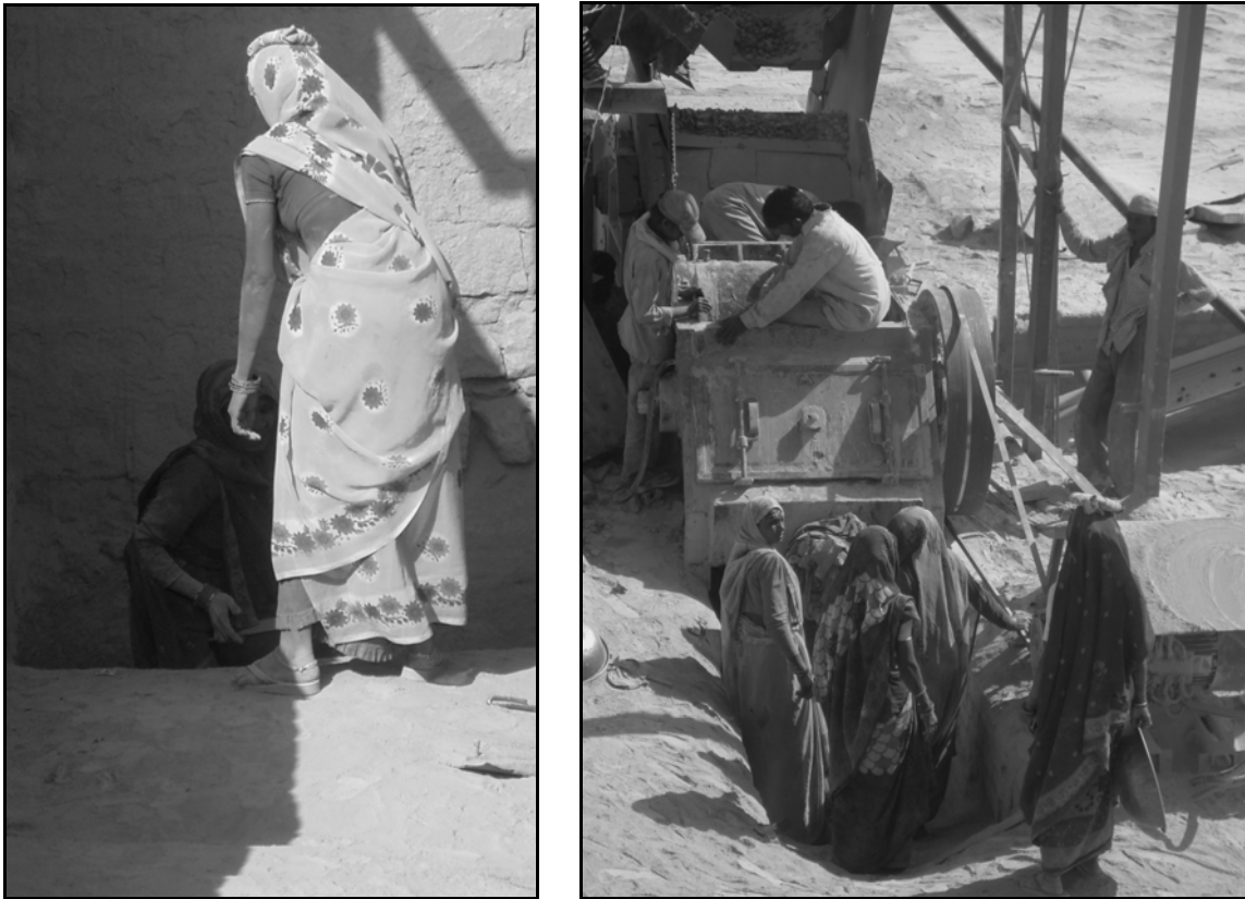
Picture 22: women cleaning dust and debris out from under the primary crusher
