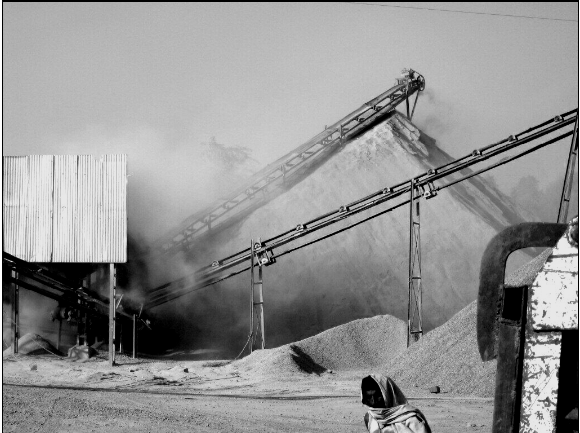
Picture 1: typical dust cloud around the crusher and sorter
