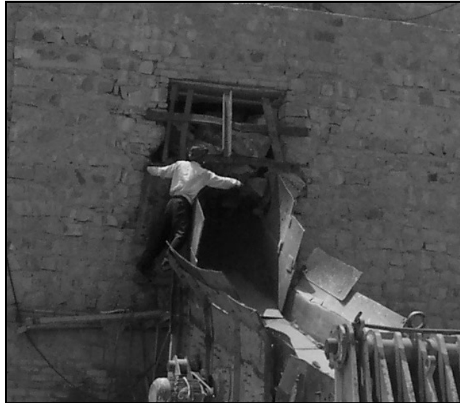
Picture 16: trying to clear and unstick the boulder chute, an extremely dangerous work
